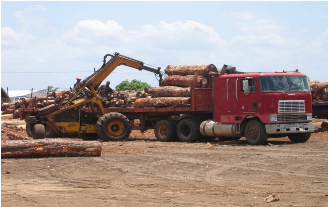
Photo 6 Timber Transport II: Mechanised loading of semi-trailer at Madeiras Alman, for transport to port at Quelimane
